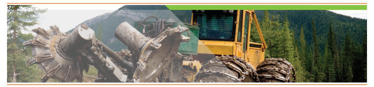
Other Pierce products include attachments for the logging industry, such as delimbers that process a cut log while a computer simultaneously measures the diameter of the log, delivering cutting instructions based on the customer's requirements. Pierce Pacific also manufactures grapples, log loaders, high speed saws, and scrap machines that move bulk materials onto or from barges. The machines characterize Pierce Pacific equipment which does more with less manpower.
